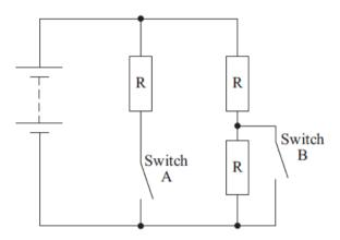
The table gives the four possible combinations of the two switches. Complete the table to show the total circuit resistance for each switch combination.
